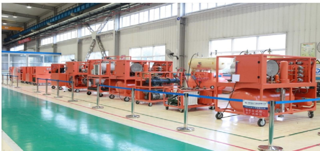
Workshop of SF 6 gas recovery unit
