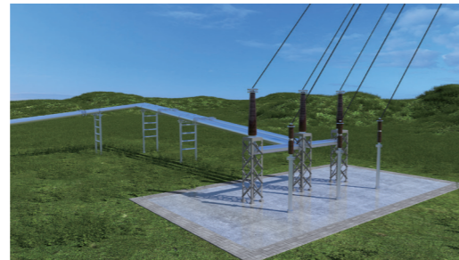
Ground overhead laying mode
