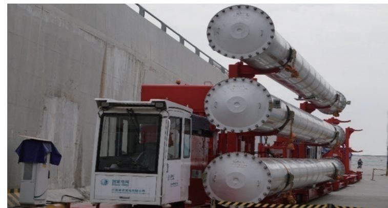
GIL tunnel transport vehicle
