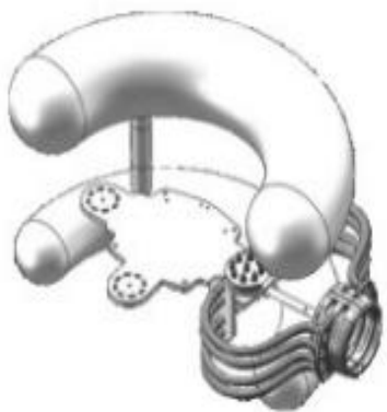
Tubular bus bar connection fittings (fixed)
