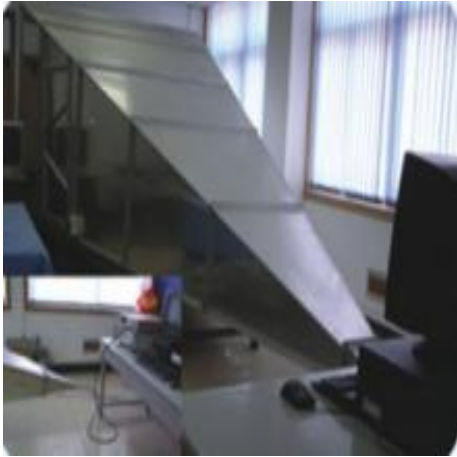
Radiated, radio-frequency, electromagnetic field immunity test equipment
